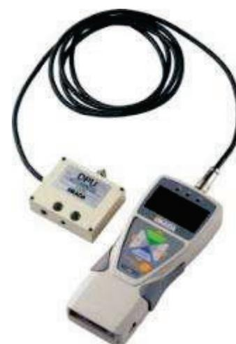
**[Load cells that can be combined with sensor separate model force gauge]**
