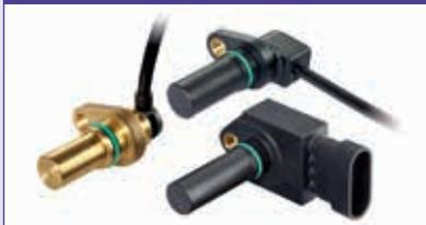
In the area of mobile operating machines and electric drives, we developed a variety of speed sensors that offer different cable lengths, connectors and insertion depths. Beside a wide temperature range, our speed sensors are either available with two frequency outputs or one frequency and one digital direction output. Therefore, both rotational speed and direction of rotation can be detected.
